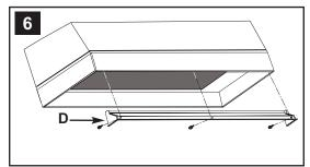
Slide the front panel section (**D**) into the nose of the custom hood base. Take care not to scratch the main liner plate when installing the front panel section of the liner. Assemble it to the cabinet using (3)  $1/2^{\circ}$  screws.
